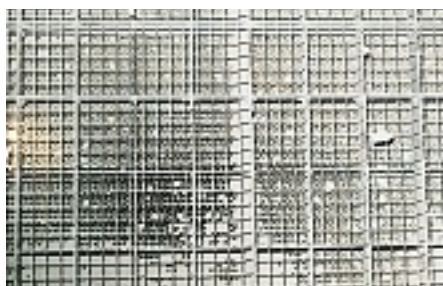
SCR, after six months process with Sonic Cleaning
