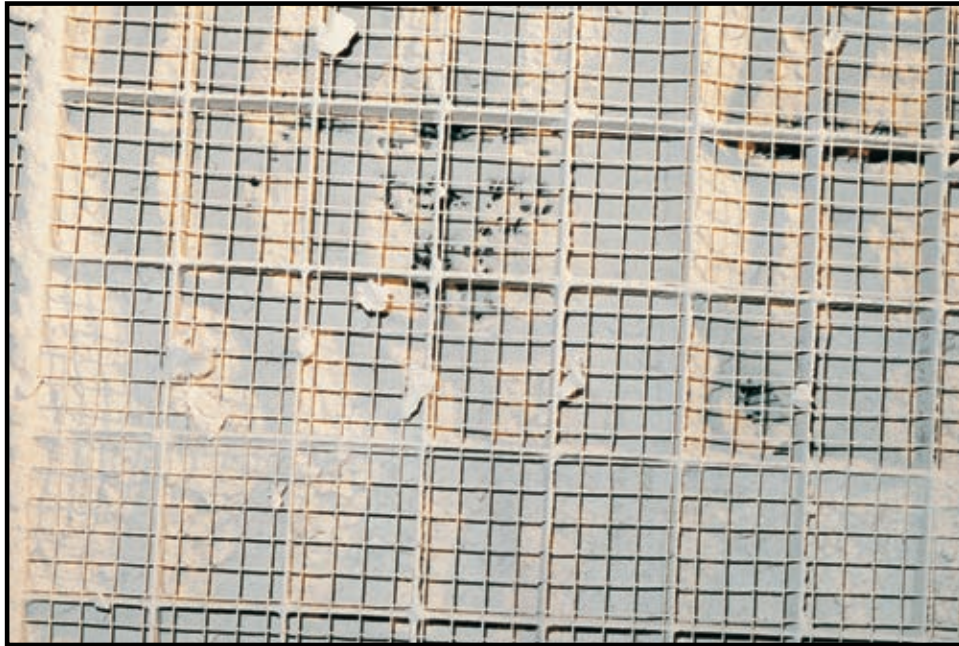
SCR, AFTER SIX MONTHS PROCESS: WITHOUT SONIC CLEANING
